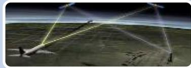
**Performance Based Navigation (PBN):** applications used when an aircraft follows a specific procedure or route within a prescribed error margin (e.g. airport approach).
